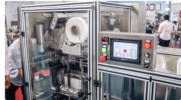
Automatic equipment cellophane box packaging in pharmaceutical production
