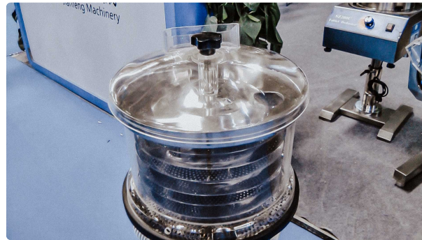
Automatic machine dust removal from tablet surface vacuum cleaner
