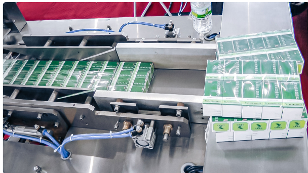
Automatic equipment cellophanator in pharmaceutical production
