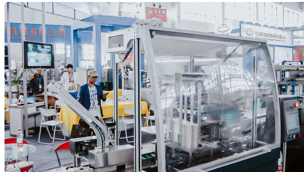
Automatic cartoning machine for packing blisters and plastic tubes into boxes CANADA
