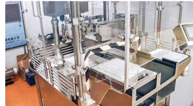
Automatic equipment for filling and closing of penicillin bottles in pharmaceutical production
