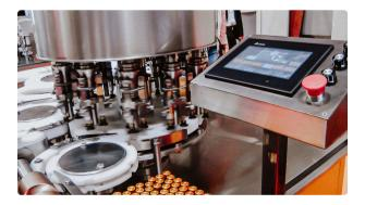
Hight speed automatic equipment for filling liquid products in penicillin bottles with... Pharmaceutical Packaging • 22.09.2020 • 9.870K views
