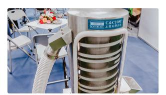
Automatic tablet polishing machine and dust removal after tablet pressing
