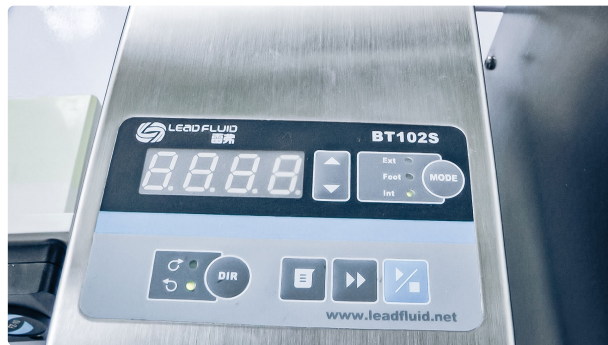
Automatic liquid dosing equipment peristaltic pumps in pharmaceutical production
