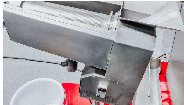
Automatic machine for removing dust from the surface of the tablets and vacuum cleaner
