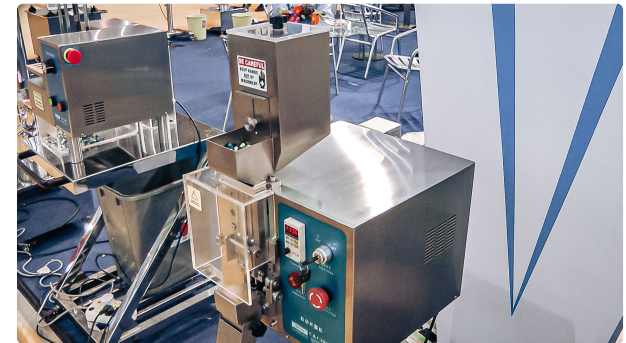
Automatic equipment for opening gelatin capsules in pharmaceutical production
