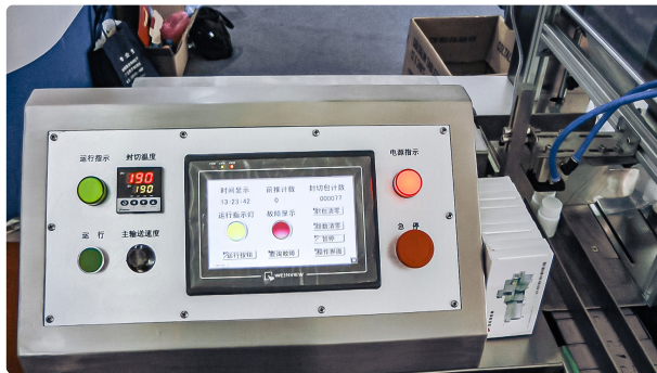
Automatic equipment group packing bottles in cellophane in pharmaceutical production
