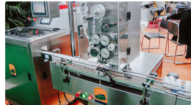
Automatic equipment for packing silica gel bags in plastic bottles with gelatin capsules
