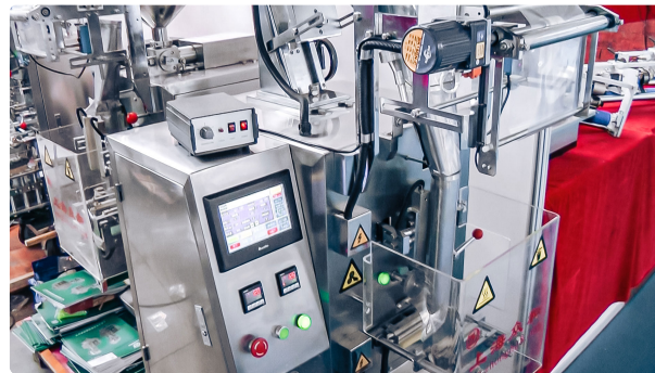
Automatic equipment for packing of products into sashet packs in pharmaceutical production
