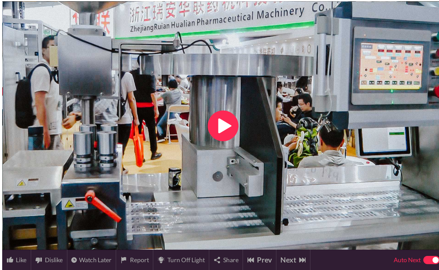
Automatic blistering machine for packing hard gelatin capsules into blister
