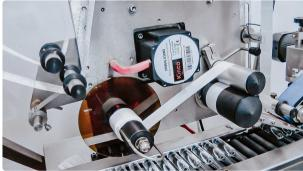
Automatic labeling machine for sticking selfadhesive labels on penicillin vials and ampoules
