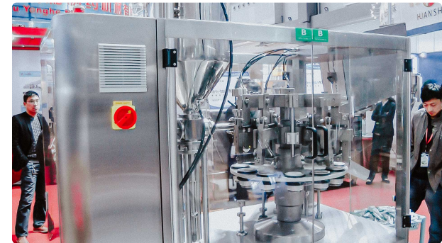
Pharmaceutical equipment for filling and sealing plastic tubes with cream and ointment
