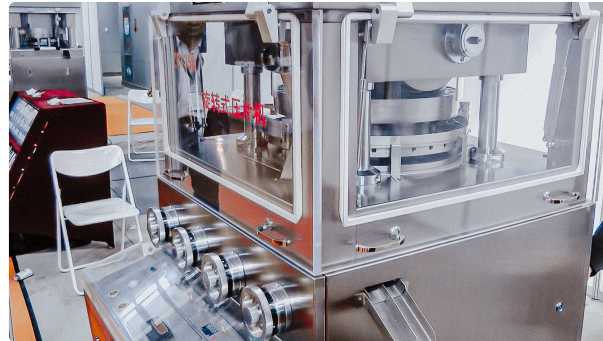
Automatic rotary tablet press for production of tablets
