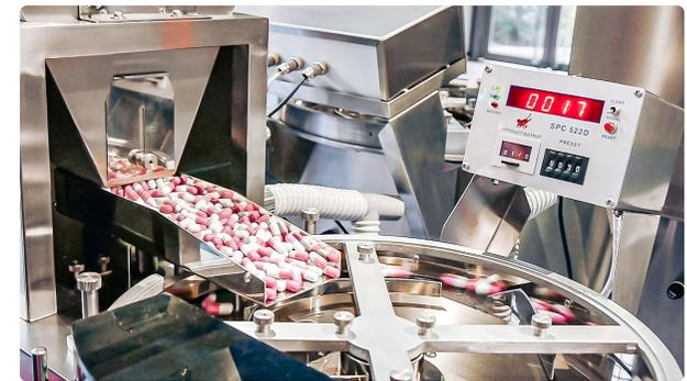
Automatic equipment for counting and packing of gelatin capsules into bottles USA
