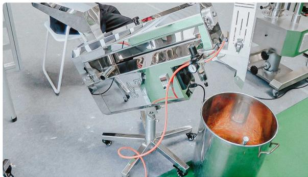
Automatic machine for polishing and dedusting hard gelatin capsules with test in metal detector
