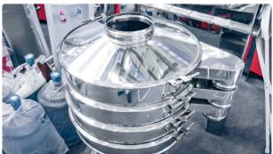
Automatic equipment for sieving powders and granules in pharmaceutical production
