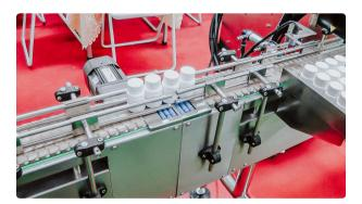
Automatic membrane induction welding machine on the neck of plastic bottle with...
