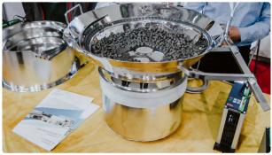
High speed machine vibration feeding rubber stoppers and aluminum cap
