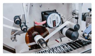
Automatic labeling machine for sticking selfadhesive labels on penicillin vials and ampoules Pharmaceutical Packaging • 25.09.2020 • 780K views
