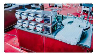
Automatic liquid filling machine for glass bottles with peristaltic pumps
