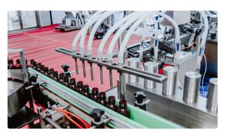
Automatic filling and capping machine for plastic medicine bottles
