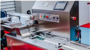
Automatic machine for packing glass ampoules in plastic containers of 10 pieces
