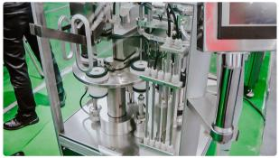
Automatic machine assembly and capping plastic syringes
