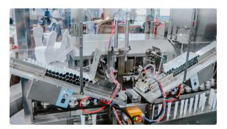
Cream, ointment and glue bottling machine for plastic and aluminum tubes
