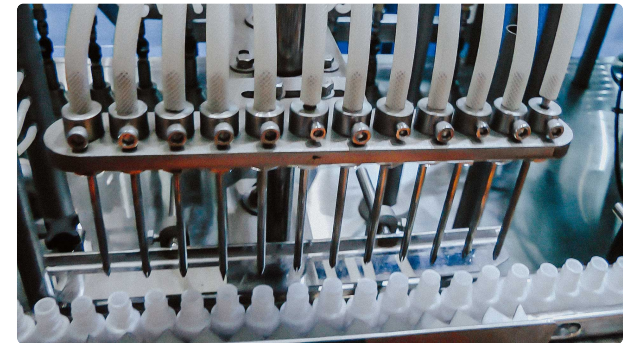
Equipment for automatic filling and capping of penicillin bottle
