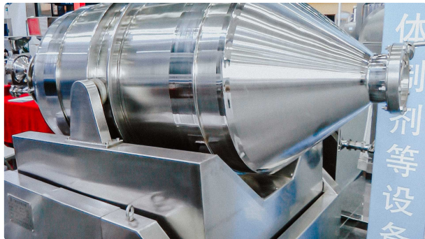
Powder mixer for food and pharmaceutical production
