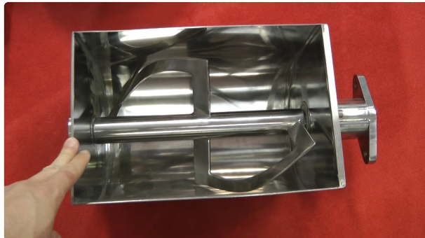
S Blade mixer for pharmaceutical laboratory drug manufacturing
