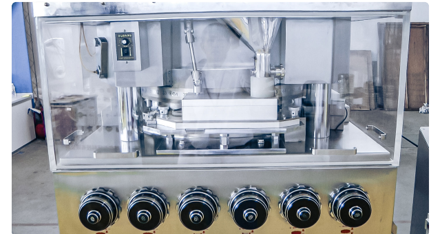
Automatic high speed tablet pressing equipment in pharmaceutical production
