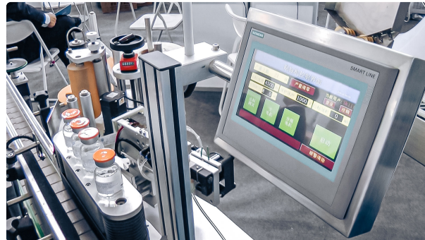
Automatic equipment for sticking self-adhesive labels on penicillin vials for pharmaceutical...
