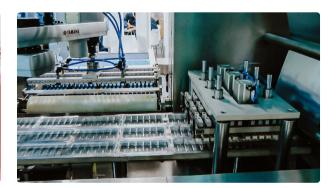
High speed automatic blister machine for PVC and ALU blister packing in penicillin bottles
