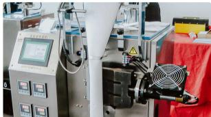
Automatic packing machine for packing powders and granules into pillow bags filter...
