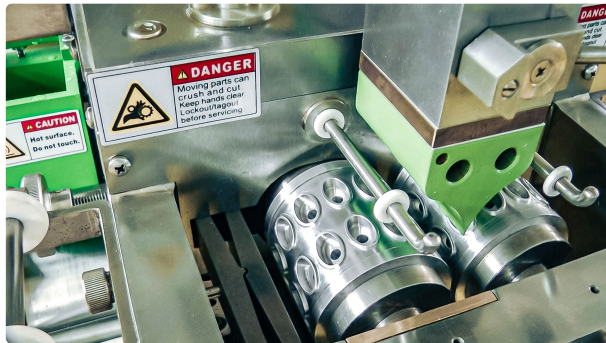
Automatic equipment for production of soft gel capsules with oil in pharmaceutical production
