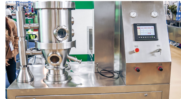
Automatic equipment for drying and granulation of powder in fluidized bed...
