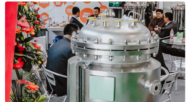
Tank for liquids volume of 200 liters with water jacket and heating for pharmaceutical liquids
