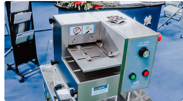
Pharmaceutical equipment for removing tablets and capsules from ready-made blisters Pharmaceutical Packaging • 17.09.2020 • 7.580K views
