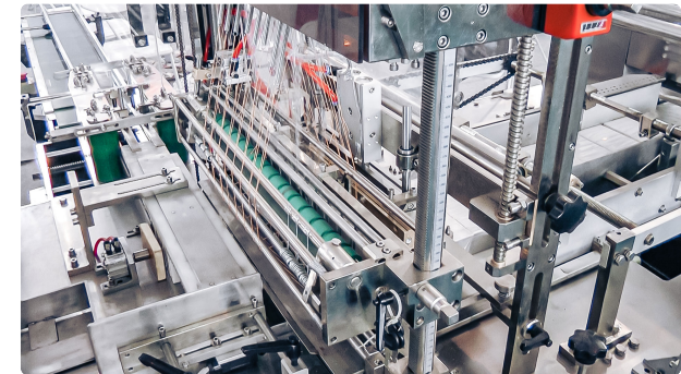
Automatic equipment packaging in cellophane film in pharmaceutical production
