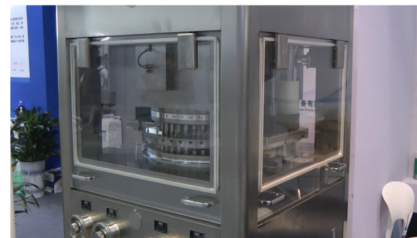
Rotary tablet press for pressing tablets of oval and cylindrical shape
