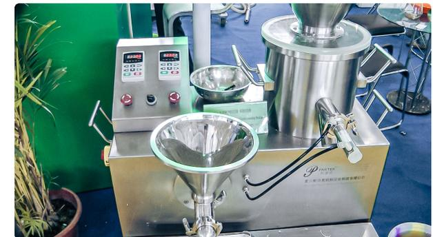
Automatic equipment for powder pelletizing by pressing through a sieve in pharmaceutical...
