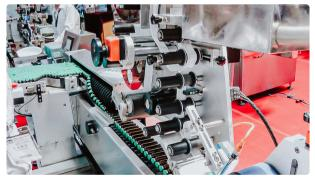
Automatic machine for packing glass ampoules in plastic containers of 10 pieces USA
