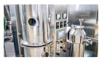
Automatic equipment for drying and granulation of powder in fluidized bed...
