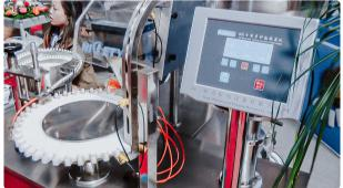
Capping and filling liquids automatic machine for pharmaceutical factory
