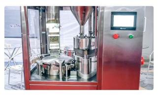
Automatic equipment for filling hard gelatine capsules with powder
