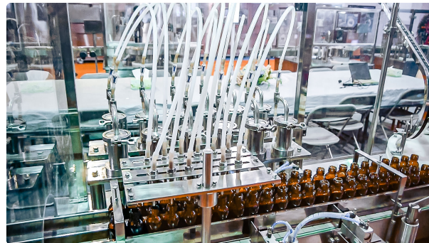
Automatic equipment for bottling medicine liquid in glass bottles and capping
