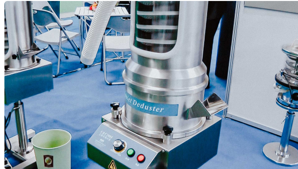
Pharmaceutical tablet dedusting machine for working with tablet rotary press
