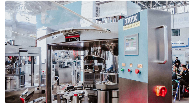
Pharmaceutical equipment for filling hard gelatin capsules with powder
