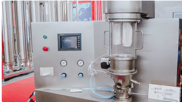
Automatic fluidized bed granulator for tablet protective coating
