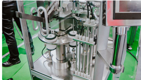
Automatic machine assembly and capping plastic syringes
