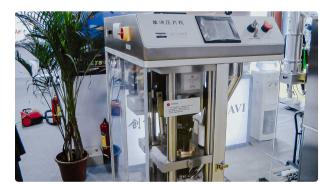
One punch laboratory tablet press for tablet pressing
