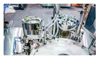
Automatic equipment for bottling and capping plastic bottles with spray nozzle
