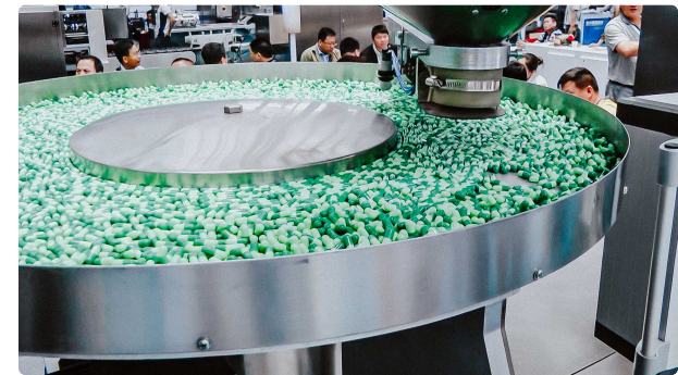
Automatic blister machine high speed for packing solid gelatin capsules into blister
