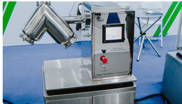
V-mixer to prepare a mixture of powders use for drug manufacture
