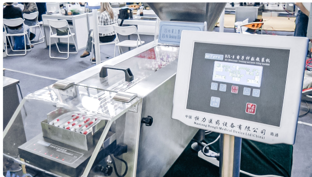
Automatic equipment for gelatine capsules counting and filling of bottles in pharmaceutical...
