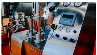
Equipment for production of pharmaceutical granules in fluidized bed granulation with...
