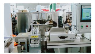
High speed automatic blistering machine for gelatine capsules blister packaging
