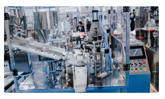
Automatic dispenser for cream and liquid filling of plastic tubes seal and release date
