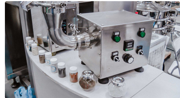
Laboratory machine granulator with powder and granule drying system
