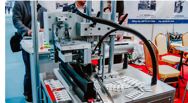
Desktop automatic machine, for soldering ultrasonic plastic tubes with cream
