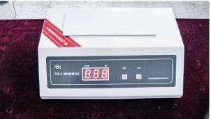
Automatic equipment for testing gelatin viscosity in pharmaceutical production Pharmaceutical Tablet Press • 08.12.2020 • 79.505K views
