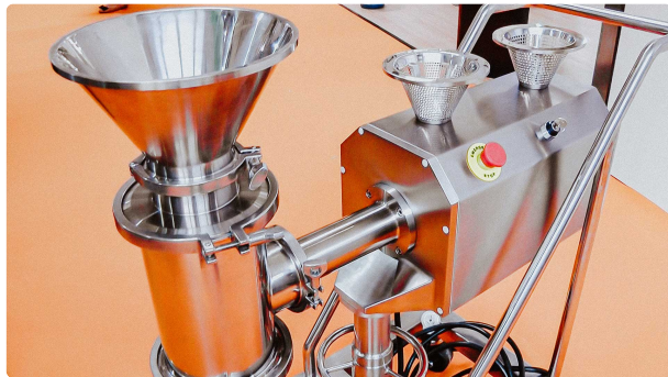
Granulator for the production of pharmaceutical granules from moistened powder
