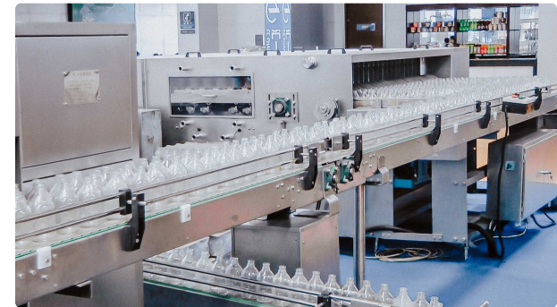
Automatic glass bottle washing machine and rinse aid in medicine filling line
