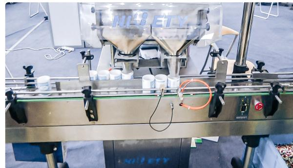
Automatic equipment for filling gelatin capsules into bottles in pharmaceutical production
