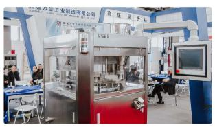
Automatic rotary tablet press for powder pressing
