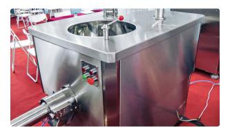
Automatic powder granulation equipment and extruder in pharmaceutical production
