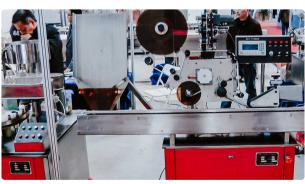
Equipment for self-adhesive labels on glass ampoules
