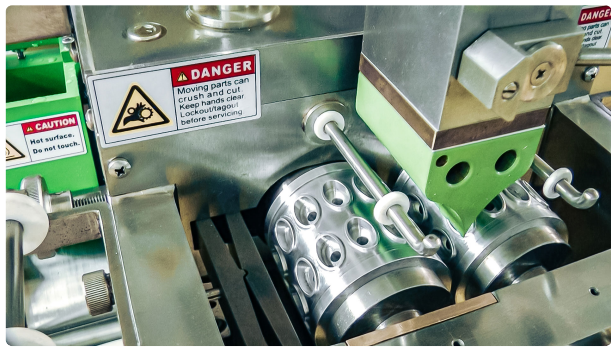
Automatic equipment for production of soft gel capsules with oil in pharmaceutical production Pharmaceutical Tablet Press · 10.12.2020 · 97.541K views
