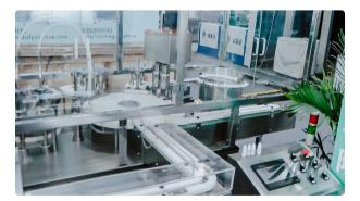
Filling and capping machine penicillin bottles with plastic cap for liquids
