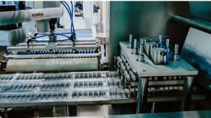
High speed automatic blister machine for PVC and ALU blister packing in penicillin bottles
