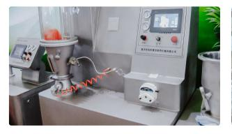
Laboratory equipment for drying and granulation in fluidized bed for pellet production
