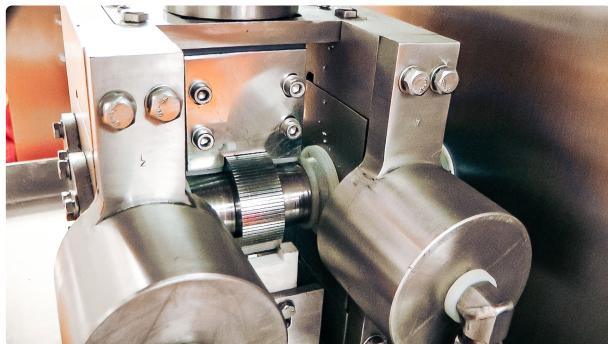
Automatic equipment for dry granulation of pellets in pharmaceutical production
