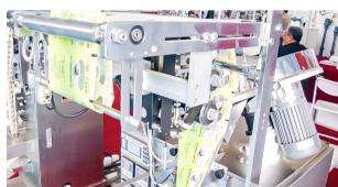
Labeling machine for sticking self-adhesive labels on top of caps and boxes
