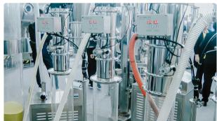
Vacuum transport system for powders for pharmaceutical equipment
